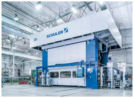
Typical of Schuler: A tension rod design servo press with 11,000 kN of pressing force. Hydraulic oil filling quantity > 5,000 L.
