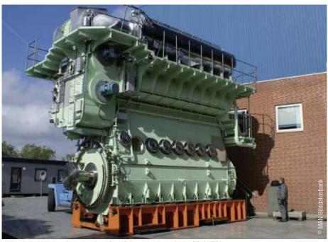
An 8-cylinder MAN 2-stroke marine diesel S35ME-B – a typical case for the OELCHECK SDA-analysis service
