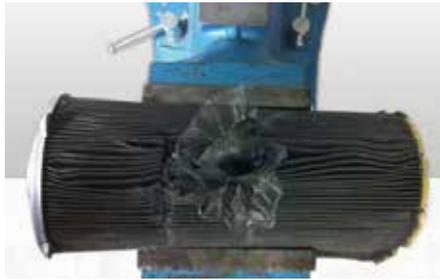
4. Now cut a representative piece of the multi-layered filter mesh (approximately 50mm x 50mm). Avoid contact with the bit of filter that has connective fabric or housing.
