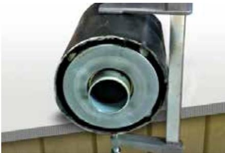
2. Locate the metal filter housing (only if the filter is built into metal housing). First unlock the casing at the flared flange. Open the sheet housing using a corner slider or an iron saw. While doing so avoid a contamination of the filter material.
