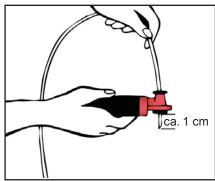
Loosen the screw and push the hose through the hole. The end of the hose should protrude approx. 1cm from the thread.
