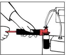
Now put the skewed-off end of the hose into the dipstick-hole or the filling hole. Always hold the bottle in an upright position. Finally pull the oil into the sample bottle by pumping steadily.
