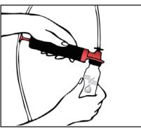
Fasten the screw in order to seal the system and screw on the sample bottle.
