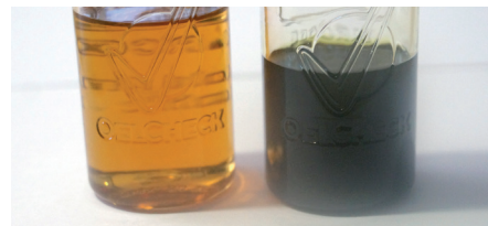
Left: fresh hydraulic oil, right: following the „diesel effect“
