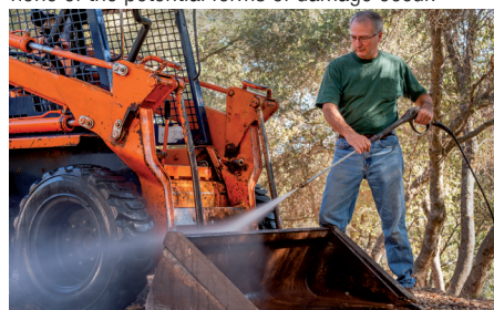
Water is one of the most common causes of damage to hydraulic systems
